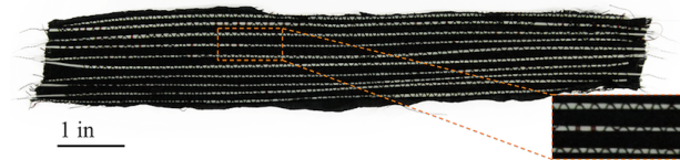
Fig. 3. Variable stiffness fibers sewn onto fabric.
