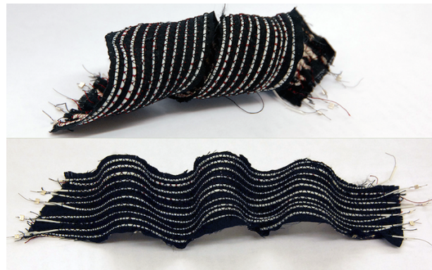
Fig. 1. Top: Variable stiffness fabric curled into a spiral. Bottom: Variable stiffness fabric shaped into an oscillatory pattern.
